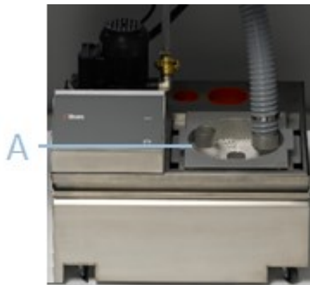
A Static filter unit
