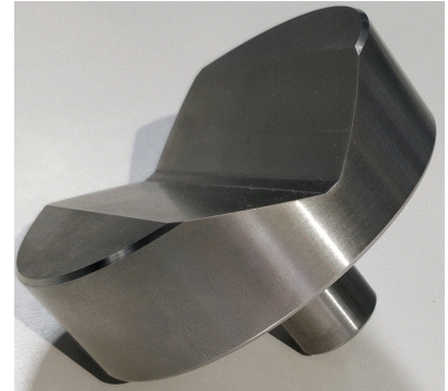
V-shape anvil for cylindrical samples (option).
